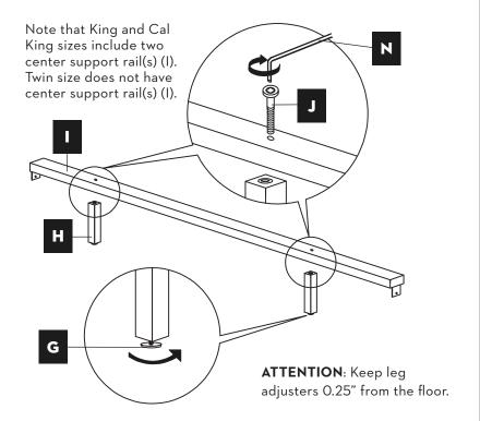
Slide center support rail(s) (I) into the head rail bracket (B) and foot rail bracket (C). Using a screwdriver, secure the center support rail(s) (I) by tightening the short screws (K) on the head rail (B) and foot rail (C)
